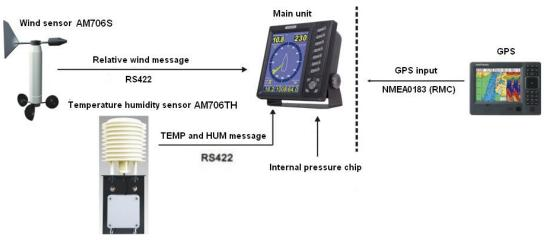
Wind sensor sends relative wind direction and speed signal (relative to ship bow and absolute value of angle signal) in digital interface format of RS422 to main unit through junction box.
