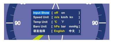
Press up/down arrow buttons for main options and left/right buttons for settings. Press [OK] to save the set values and exit or automatically save and exit without operation in 10s.
